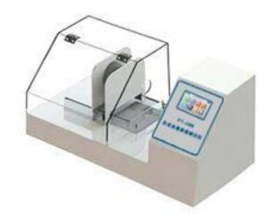
0002n / m at a distance of 30.5cm from the center of the sample to the target area of the tested sample horizontally from the needle tube with an inner diameter of 0.84mm at a pressure of 16kpa. Remove it for visual inspection within 10s.
